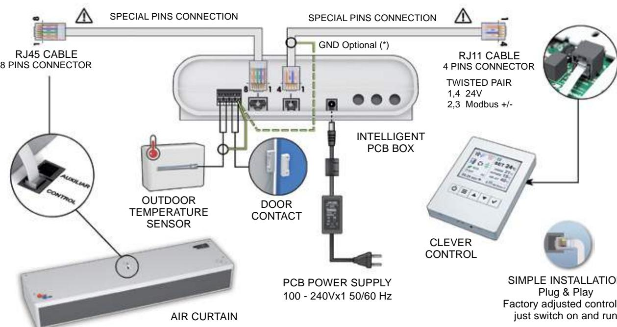
(\*) If there are communication issues (interferences), use shielded cable connected to GND
