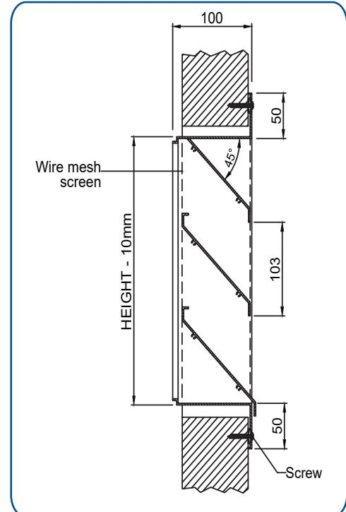
>> The exhaust air louver is composed of a set of blades made of 2MM aluminum extruded profile/ GI sheet arranged in 45 degree in horizontal rows and inclined downward to protect against rain water.
