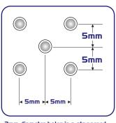
3mm diameter holes in a staggered pattern
