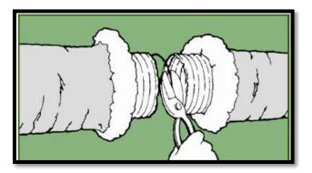
1) After desired length is determined, cut completely around and through duct with knife or scissors. Cut wire with wire cutters. Fold back jacket and insulation.
