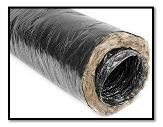
**SUPER VENT SV-IFDM** model is made with double laminated metallized polyester clear film bonded with strong adhesive permanently to the corrosion resistant steel wire helix. Thermal efficiency is provided by wrapping the exterior with Ecose technology fiberglass insulation. Strong vapour barrier is made with metallized polyester film laminate.
