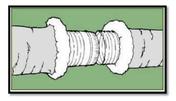
1) Fold back jacket and insulation from core. Butt two cores together on a 4" [100 mm] min. length metal sleeve.
