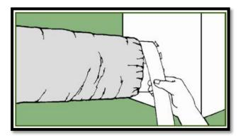
3) Pull jacket and insulation back over core. Tape jacket with at least 2 wraps of duct tape. A clamp may be used in place of or in combination with the duct tape.
