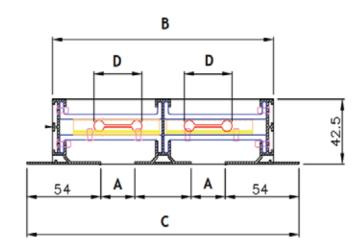
C) FLOW BAR DIFFUSER (FBF - Flush Type Flow Bar Diffuser) 41 mm Flange
